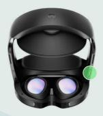
You can turn the volume up and down with this button, located on the right underside of the headset.
