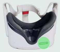
You can turn the volume up and down with this button, located on the right underside of the headset.
